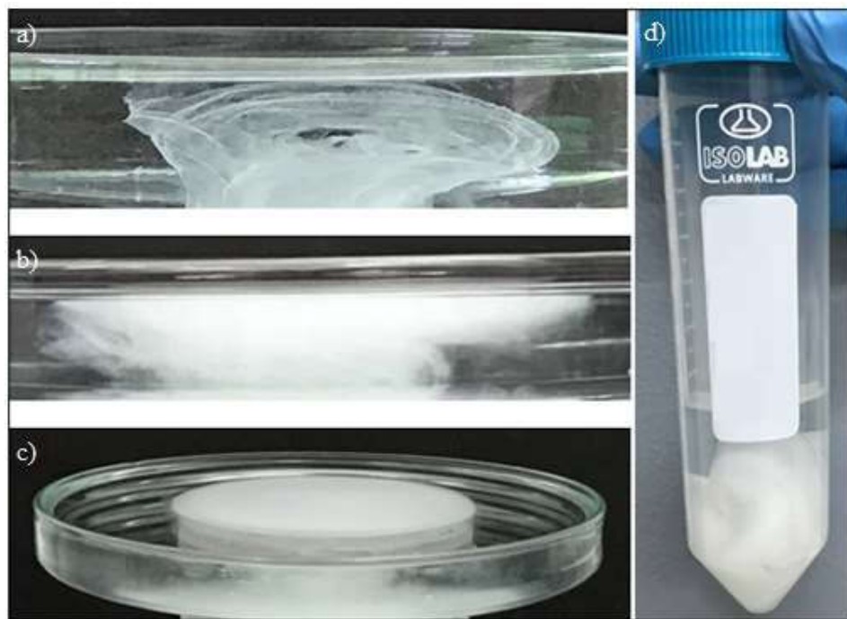
Figure 3.2. PHBV/PCL scaffold formation in an ethanol bath, during (a and b) and after (c and d) electrospinning.
