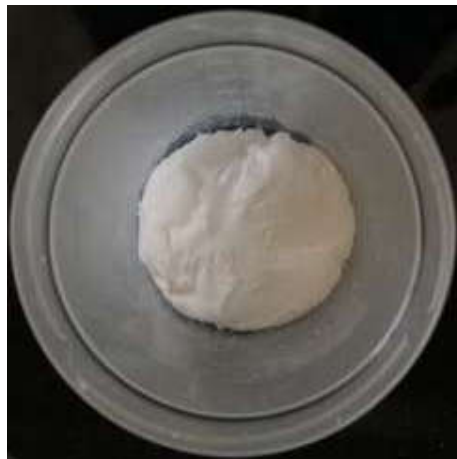
Figure 3.3. PHBV/PCL wet electrospun scaffold after drying
