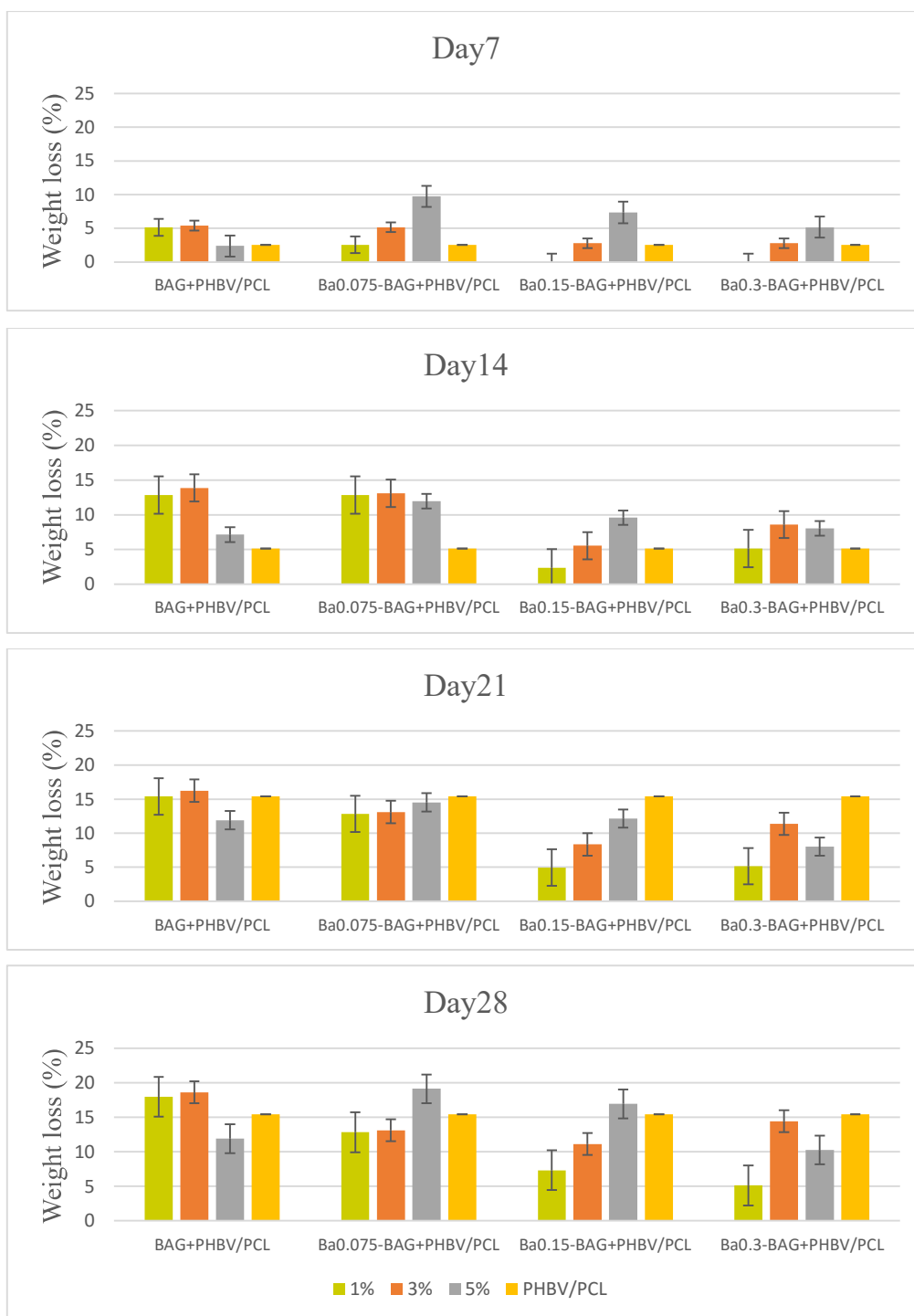
Figure 4.6. Total weight loss of scaffold groups after different PBS (0.01 M, PH: 7.4, at 37 °C) incubation periods.
